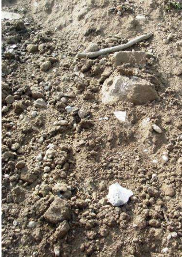
Incoming C&DW material
